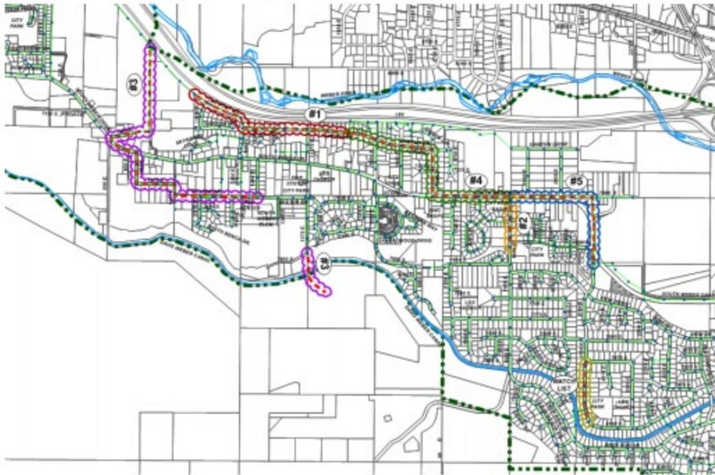
Since pipes come in standard sizes, a pipe upsized to accommodate future growth may contain excess capacity. For example, a 10-inch pipe is required to convey the sewer discharge from 400 homes (ERUs). However, a 10-inch sewer line has the capacity to serve about 500 ERUs; therefore, there are 100 ERUs of excess capacity in that 10-inch sewer line.
