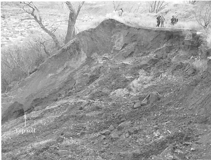
Figure 6. View to the southeast showing landslide main scarp and fill placed on the upper slope. Near the left edge of the photo, black top soil at the base of the scarp (arrow) underlying the brown fill is evident and indicates the original slope surface.
